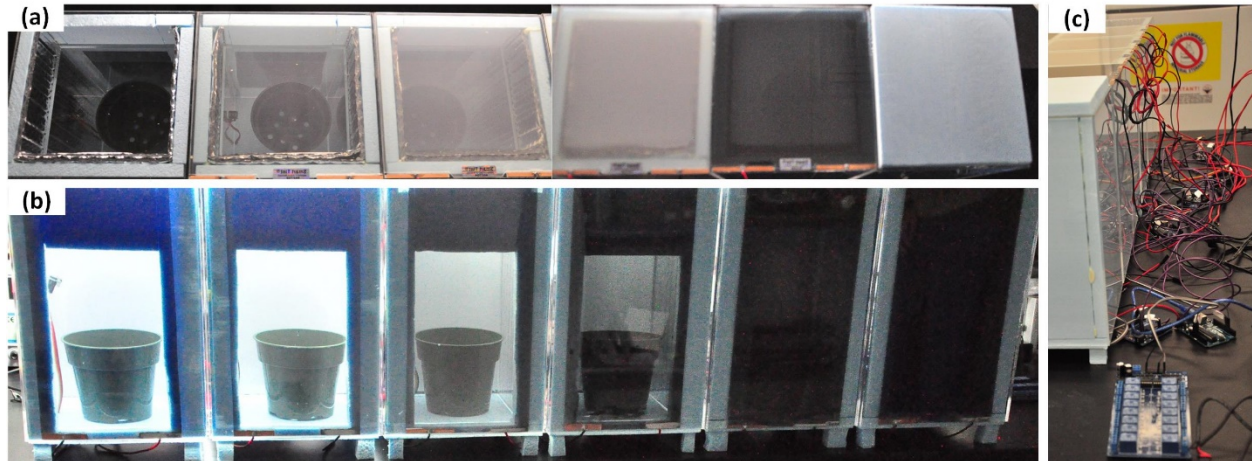
Figure 4.7 Improved miniature greenhouses (a) the top view, (b) the front, and the circuits behind the greenhouses.
